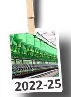
Spinning Capacity increased by greenfield expansion with installation of 12K+ spindles at Ludhiana (2<sup>nd</sup> unit) for manufacture of synthetic yarn. Present installed capacity-65K+ spindles
